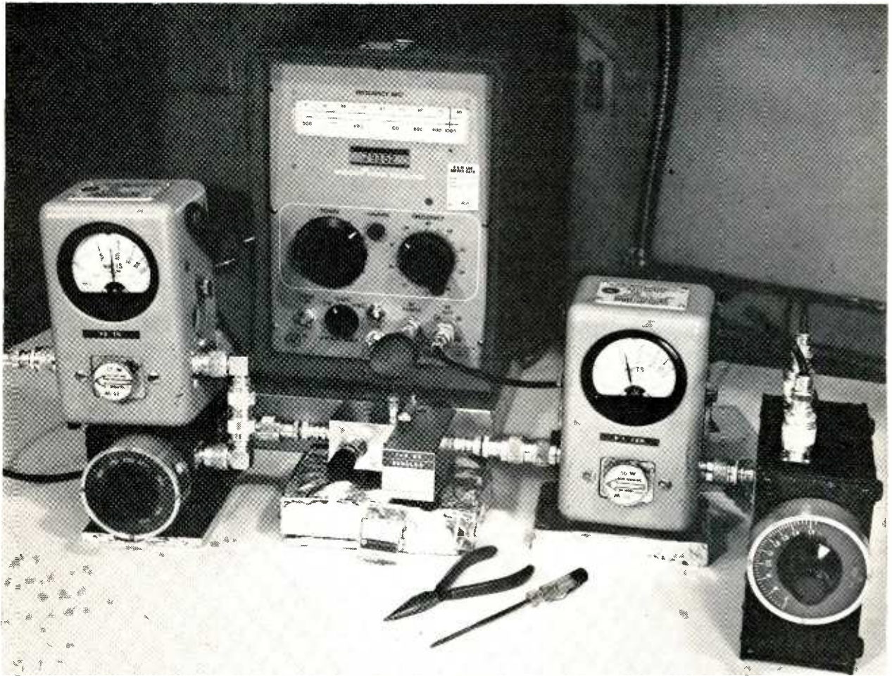
Test arrangement for 1-to-2-Gc doubler includes a wattmeter, at left, indicating the input power of 12 watts; a power oscillator set at 1 Gc; and another wattmeter, at right, showing the power output level of 7 watts at 2 Gc.
