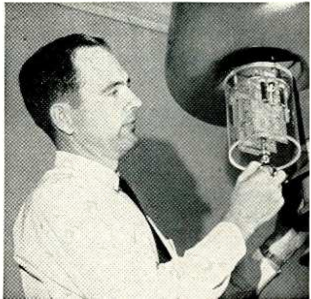
Plugging coder electronics into the head of a Traser system prior to prototype testing. Heavy magnetic shielding surrounds encoder unit to assure that passage of line current and resulting magnetic fields do not affect coder output accuracy appreciably.
